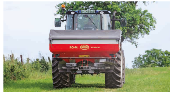
One-sided boundary spreading - spreading from the border with the border spreading plate
