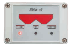
Indicates which border spreading device is active
