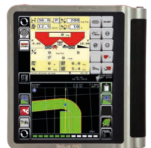
Automatic RPM warning on the terminal
