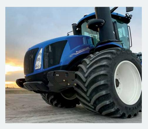
When equipped with LSW1250/35R46 singles, the overall width measures about 150 inches or 12.5 feet. This narrow roading width, in combination with a light footprint, provides a middle ground when choosing between SmartTrax and high-flotation duals.
