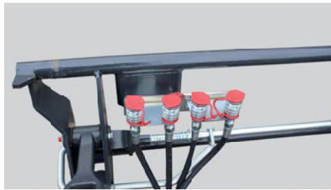
3rd and 4th control circuit (here as a plug-in coupling) For easy handling of hydraulic implements like the bucket with grapple, grip fork or bale lifting fork.
