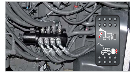
Comfort Hydraulics • Selector switch for the activation of front loader or rear hydraulics; a simultaneous double occupancy is excluded.
