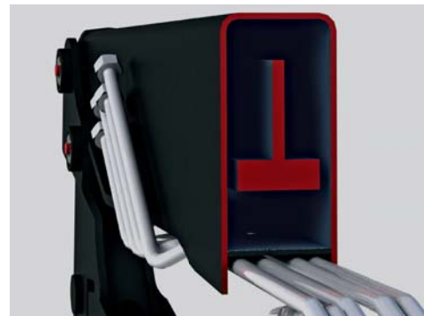
Cross section of a loader arm – the control rod is in the cavity, below are the hydraulic lines.
