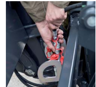
3 Plug in the hydraulic connection
