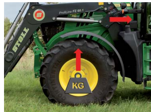
The attachment components are close to the driver's cab – which reduces the workload on the tractor's front axle.
