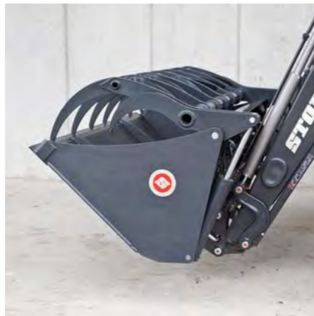
2 Tilt the implement – the locking mechanism engages automatically
